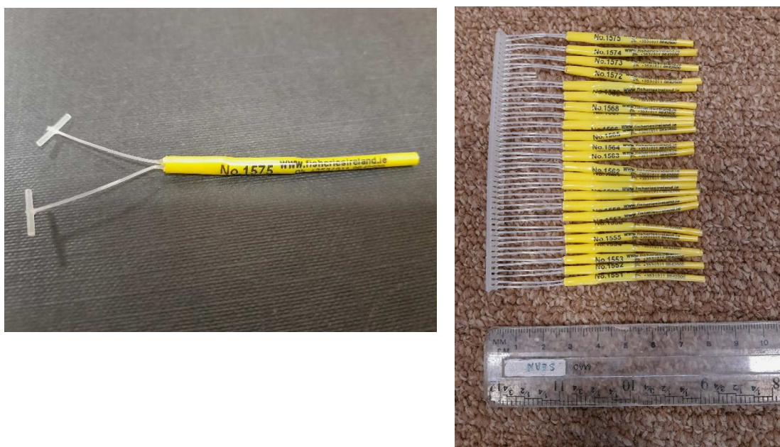
Fig. 1. Double anchor T- bar PIT tag (DTBA-PIT) used for shad. PIT tag enveloped by tag body.
